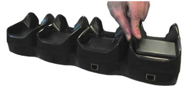
Figure 5 - Spare Battery Removal
